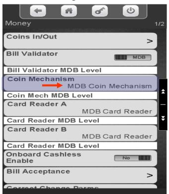
Touch the desired Coin Mechanism option and press Done to save.
