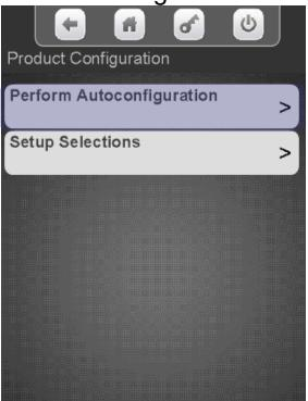
Touch Start Autoconfiguration and the controller will scan all the motors and automatically enable all motors that are detected.
