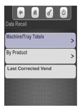
The display will show resettable & non resettable SureVend ™ corrected totals by Machine and Tray
