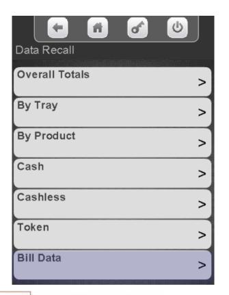
This Screen below allows you to view information about bills by denomination, both accepted and paid out when using a validator or recycler. Also included is the current value of bills stored in a recycler cassette.
