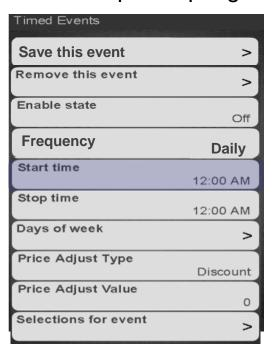
Touch the arrows key above and below the hour or minutes to change the time. Touch the AM/PM to toggle. If 24 hour clock was selected in the Time/Date menu under System Settings AM/PM will not appear.
