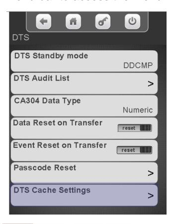
This setting enables or disables the ability of the Atlas board to prepare a new DEX file every 5 minutes and have it available on demand for quicker DEX reads required for non-Crane telemetry devices.
